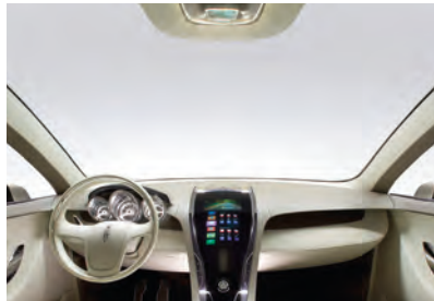
Lincoln concept car with Exatec® Lexan* PC resin offers lightweight durability and weathering performance to glass-like abrasion resistance and optical appearance.
